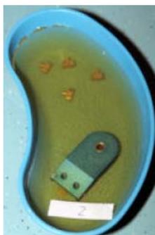
Figure 1. Aluminum and brass material embedded in glycerol gelatine (DAB 9) for artefact diagnostic
